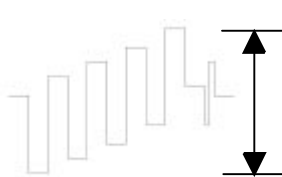
Fig. 20 Signal Pb Pin 3 of Connector P0YU ; 1Vpp
