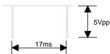
Fig. 18 Vertical Sync Signals TP5854
