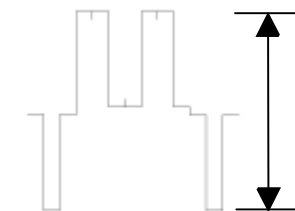
Fig. 3 Signal R Pin 5 of Connector P0YU : 1.4Vpp TP5706 ; 1.8Vpp
