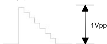
Fig. 14 Signal RGB Pins 1, 3, and 5 of connector P0PC
