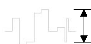
Fig. 21 Signal Pr Pin 5 of Connector P0YU ; 1Vpp
